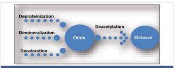
Figure 3: The processes of chitosan production from crustacean shells.
