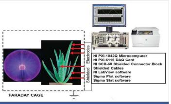
**Figure 1:** Diagram of the experimental setup for detection of electrical plant responses induced with a plasma ball. A similar experimental setup was used for experiments with the Venus flytrap [8].
