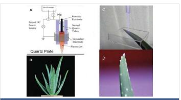
Figure 7: Treatment of *Aloe vera* leaf with a cold He-plasma jet separated by a thin quartz plate. (A) Cold atmospheric pressure He-plasma jet above a quartz plate; (B) *Aloe vera* plant; (C) Treatment of *Aloe vera* leaf with cold He-plasma jet covered by a thin quartz plate from an optical cuvette; (D) *Aloe vera* leaf after 100 minutes of treatment in the setup shown on the panel (C).
