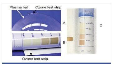
**Figure 2:** (A, B): Testing ozone production during 10 minutes exposure of to the ozone test strip near the surface of the plasma lamp. (C): Test of the ozone concentration after 10 min exposure to CAPPJ.
