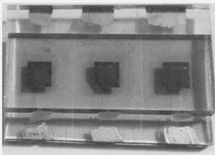
Figure 2: DSSC sensitized with hydrolyzed chlorophyll as dye.
